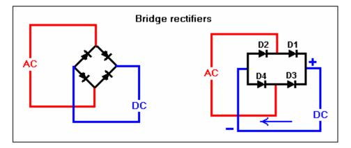
Diodes may be a bit confusing, but they are only a one-way valve that has the + current flowing in the direction of the `arrow'. Simply put, positive current flows from right to left in the above diagram. Alternating current, however, moves back and forth, thus the diodes will block current flow in one direction each way, only allowing a half-wave + to pass into the DC circuit at any one time.
