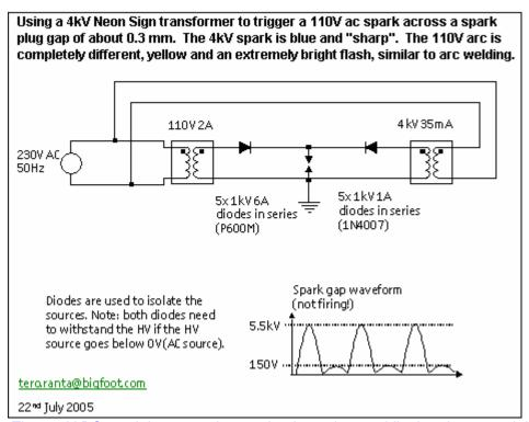
The 110V DC spark is not continuous, but intermittent, while the trigger spark is continuous. Using higher frequency (e.g. modified inverter for example) and perhaps higher voltage (250V DC) should help to get the 110V DC firing more consistent.
