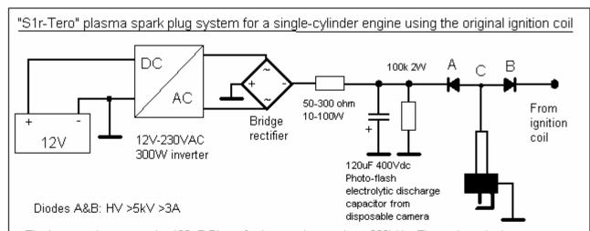
The inverter charges up the 120uF Photo-flash capacitor to about 300Vdc. The resistor (or lamp or an inductor) is used to limit the charging current to the capacitor. The polarities of the bridge rectifier, capacitor and two diodes are reversed, because it seems that the engine's ignition circuit gives a better spark in the negative direction.
